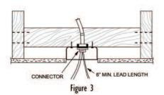
outlet box for ease in making connections. See Figure 3. Wires should be spread apart with the grounded conductor and equipment-grounding conductor on one side of the outlet box and the undergrounded conductor on the other side of the outlet box. After the splices have been made, they need to be turned upward and carefully pushed up into the outlet box.
